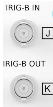
Figure 23: IRIG-B input [J] and output [K] connectors
